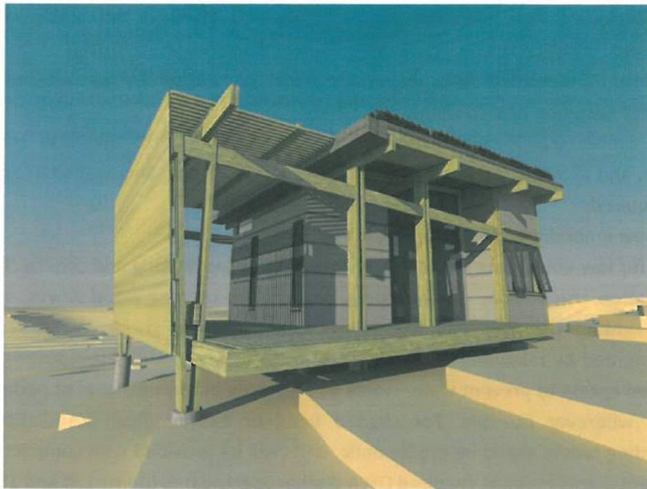
Figure 5.12: 3-D rendering of proposed new cabin (item 15), showing low footprint timber-frame construction, and visual mitigation.
