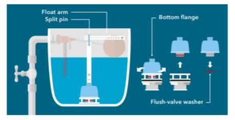
IIP: Different manufacturers use different mechanisms. To ensure that you get the correct replacement washer, take your existing old washer along when visiting the hardware store.
