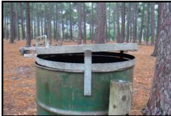
Figure 13. Alleged baboon proof lid which, although heavy to lift up, is not a deterrent for a raiding baboon.
